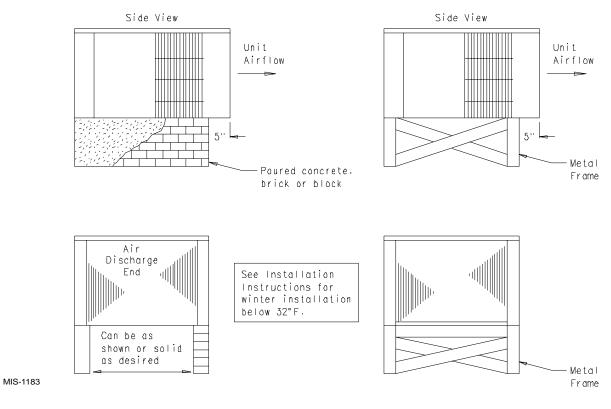
FIGURE 4 AIRFLOW and SERVICE ACCESS CLEARANCES
